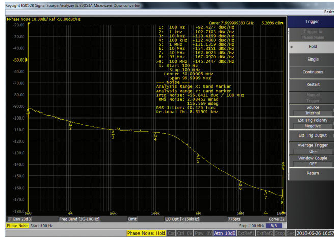
Figure 2. RMS jitter: 8.0 GHz.
