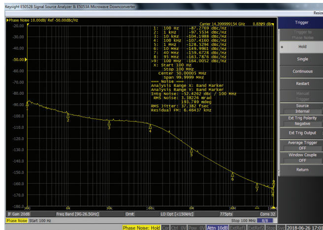
Figure 3. RMS jitter: 14.4 GHz.
